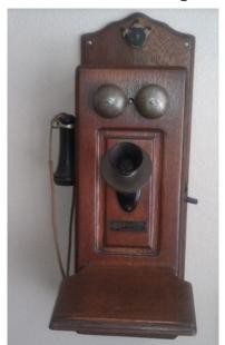
The phones used were of the type shown in the first picture. They were wooden boxes with a crank to ring with. They had to be maintained with batteries. They were large one and a half volt batteries.
